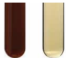
Brake fluid before and after service
