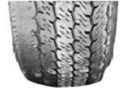
Signs of irregular tire wear
