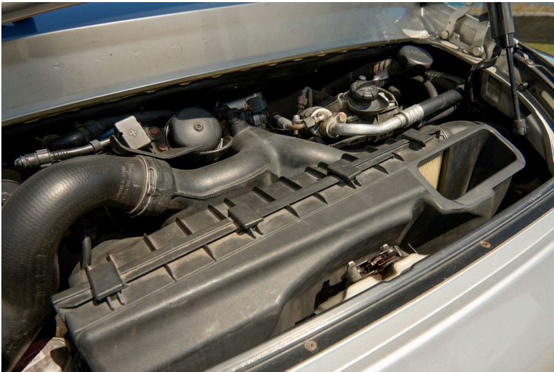
Thalmann aims to push the twin-turbo 3.6-liter flat six-cylinder engine to a million miles and beyond.
