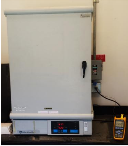
Figure 9 – The low temperature oven's internal thermometer varies by a considerable amount. A more accurate thermocouple is used to measure temperature during heat treatments.
