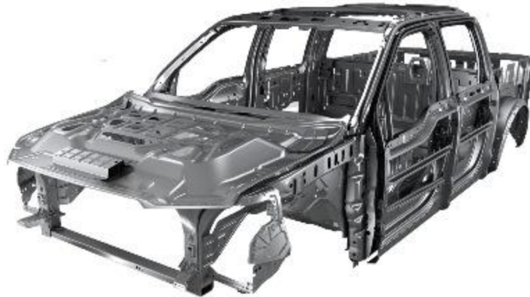
Figure 1 - The new 2015 Ford F-150 body is made entirely of extruded aluminum. The benefits in transitioning from steel include better corrosion resistance, a better strength-to-weight ratio, and a 700 pound reduction in vehicle weight. 1
