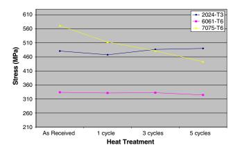
Fig. 8 Ultimate strength for all alloys after high heat treatments, at 205  $^{\circ}\mathrm{C}$
