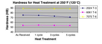
Fig. 9 Hardness for all alloys after low heat treatments
