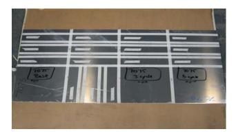
Fig. 3 Marked rectangular samples on uncoated sheet
