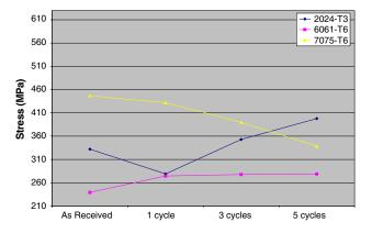
Fig. 6 Yield strength for all alloys after high heat treatments, at 205  $^{\circ}\mathrm{C}$
