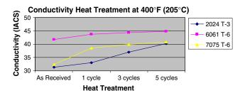
Fig. 12 Conductivity for all alloys after high heat treatments
