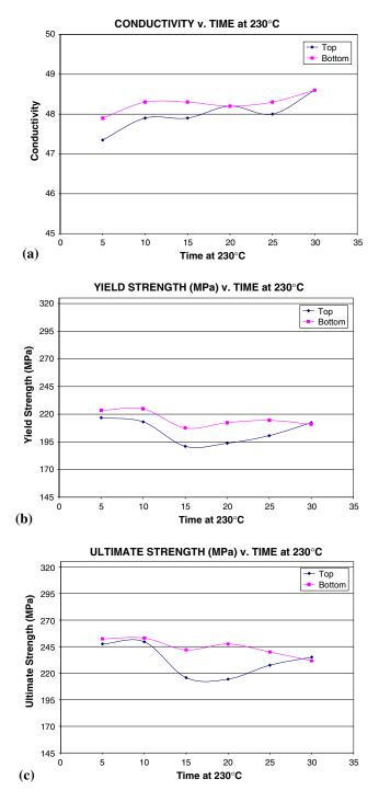
Fig. 2 (a) Conductivity (%IACS), (b) yield strength, and (c) ultimate strength for 6061 aluminum at 230  $^{\circ}$ C (time in minutes)
