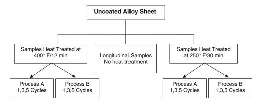
Fig. 4 Organization of uncoated samples for all three alloys heat treating and testing
