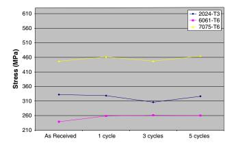
Fig. 5 Yield strength for all alloys after low heat treatments, at 120  $^{\circ}\mathrm{C}$
