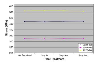
Fig. 7 Ultimate strength for all alloys after high heat treatments, at 120  $^{\circ}\mathrm{C}$
