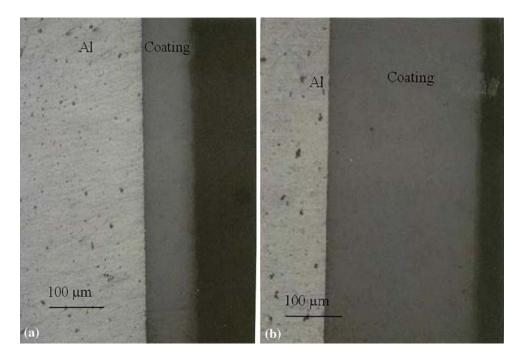
Fig. 16 Varied coating thicknesses of 2024-T3: (a) low-temperature cure and (b) high-temperature cure
