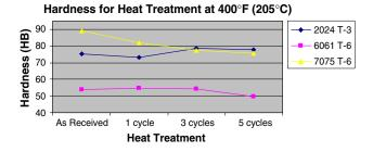
Fig. 10 Hardness for all alloys after high heat treatments
