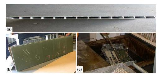
Fig. 1 (a) Cross-sectional view of Marine Corp AM2 mat, (b) as-received landing mat, and (c) tensile samples being removed from oil bath
