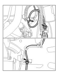
4. Press the lead into the holders by pressing on the rubber sleeves **-arrow-**.
