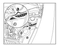
7. Cut through the fabric tape in the radiator tank, in the area -a-, and expose the remaining ABS lead.
