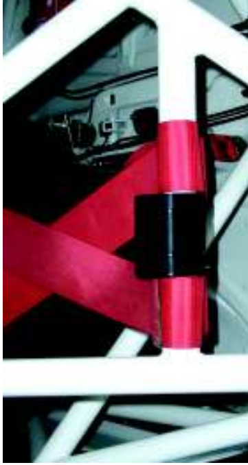
example for a spreader using FIA 8857-2001 padding material
