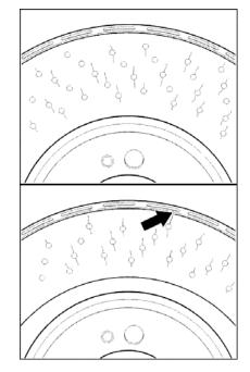
C. Brake disc with torn friction plate rim -arrow-.
