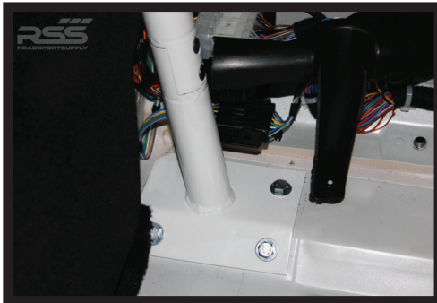
Front Legs Bolt To Floor Underneath Carpet Note: Subtle Notching of Carpet Required
