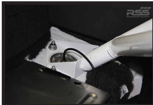
Rear Extensions Bolt To Rear Shock Towers Note: Subtle Notching of Carpet Required
