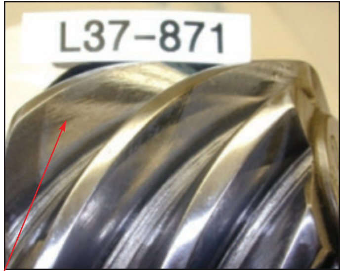
Pinion gear - original machine marks still present.
