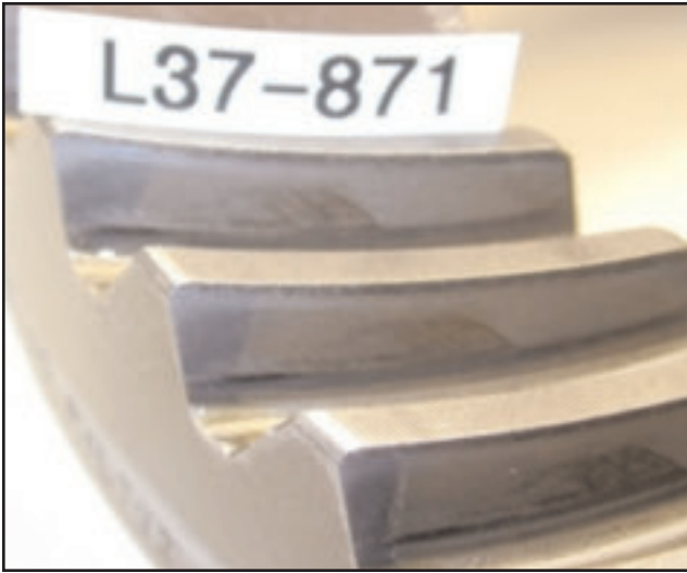
Ring gear exhibits very low wear.
