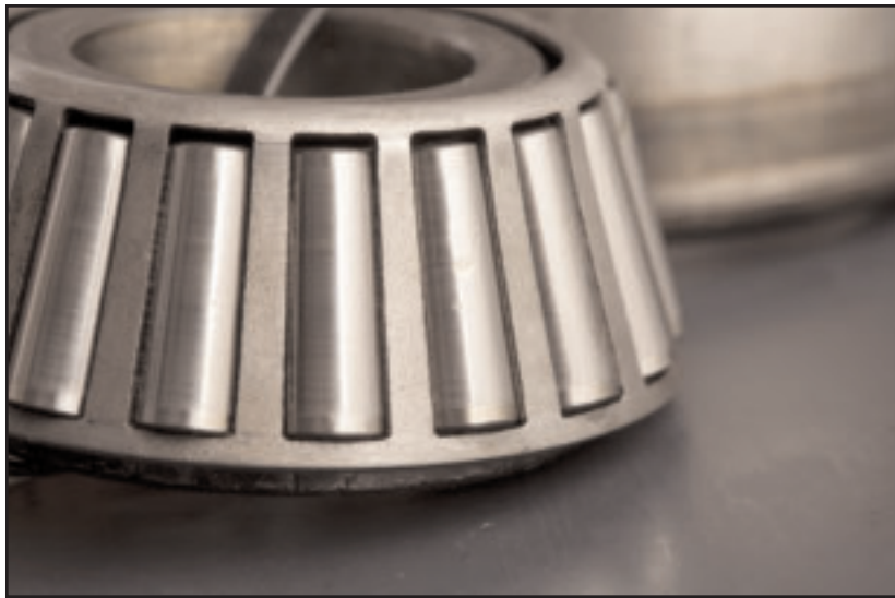
Pinion tapered roller bearing in like-new condition.
