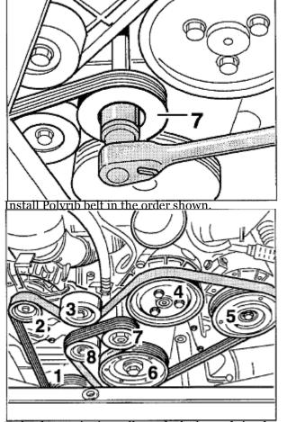
Twist the tensioning roller 7 clockwise and simultaneously place the belt on the idler pulley 8. Subsequently relieve the tensioning roller slowly. Visually check whether the belt is correctly positioned on all pulleys.
