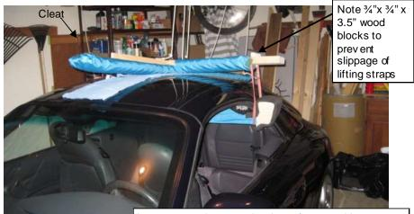
Lower cross piece onto hard top. (protect with microf iber towels if desired.) Place yoke inside car. Attach yoke to cross piece with lifting straps. Yoke pads should contact "shirt hangers" inside hard top. Disconnect hard top from car.
