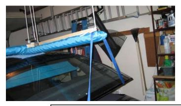
I added a stabilizing strap to the back after lifting the hard top clear of the car. The strap does not take much load, but keeps the hard tof rom rocking. The strap is attached to the hold-down cams under the hard top.
