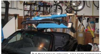
Pull lifting rope to raise top. Use angle control rope to tilt hard topf or easy disengagement from windshield. It takes about 30 lbs. of force on the rope to raise the top. Minimal force on the angle control is needed. CAREFULLY tie off to the cleat.
