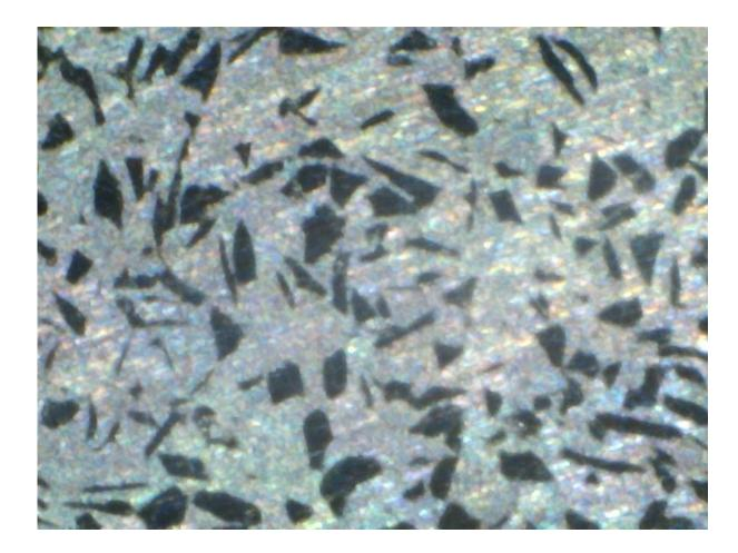
(6) In Alusil (944, 968, Gen 2 etc) the whole block is cast with a mixture of silicon particles that emerge evenly out of solution as the casting cools forming securely entrapped evenly distributed surfaces – but it is therefore very hard to machine all over the block - and therefore expensive to manufacture.
