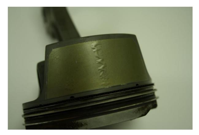
One other observation needed exploring – we were getting more Tiptronics with scored bores than manuals (despite less sold) but if we were right that it was particles penetrating oil film thickness causing scoring – that fits because the slower the revs the more time there is to squeeze out the oil film in one cycle and the higher the thrust loads the quicker they will reduce the film thickness – and Tiptronics naturally pull away in  $2^{nd}$  and under higher torque – so that fitted perfectly.
