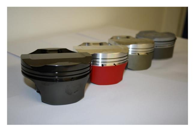
(18) The piston we had coated in "**Diamond Like Coating**" revealed the answer because the very thin coating on most of the thrust face was still
