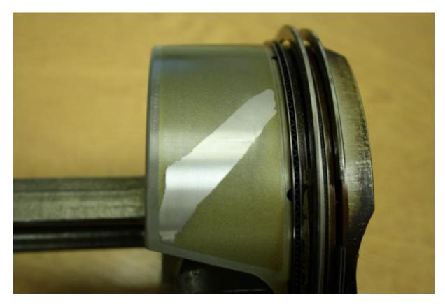
The last is by far the best showing how despite still being in tact with adjacent coating it has bubbled away from the piston – but still running OK against the
