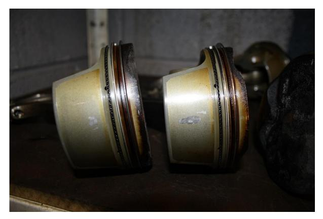
If it was silicon still bonded to the bore that plucked out the coating then the loss would extend up and down the piston at this stage while these pictures demonstrate the temporary nature of the particle release.
