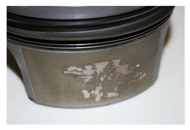
The next picture shows poor coating bonding.
