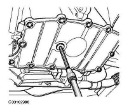
Fig. 28: Identifying Oil Drain Plug - As Of MY 2002 Courtesy of PORSCHE OF NORTH AMERICA, INC.
