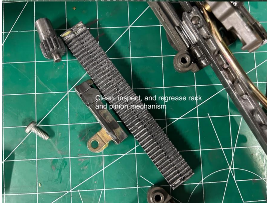
Disassembly and inspection of central drive mechanism on the bench.
