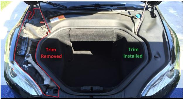
To access the top of the headlight and the vertical adjusters the 2 large plastic trim panels on either side of the frunk must be removed.
