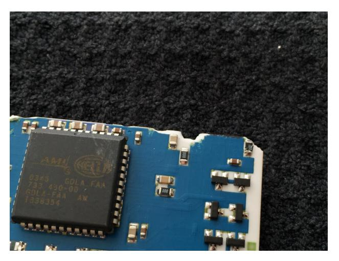
This picture shows the damage that can happen when using pliers to remove the board,
