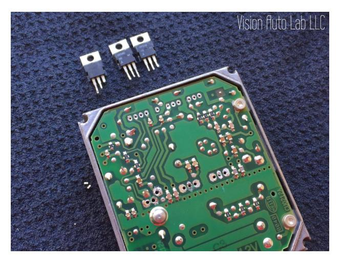
Next desolder and remove the original MOSFETs. Replace these with the IRF1405 (x1) and FDP3682 (x2) in the proper locations, IRF1405 will go into the position with the staggered pin location, FDP3682s will occupy the other locations with the pins locations in-line.
