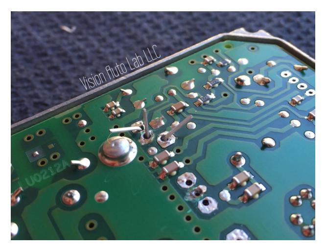
TIP: Once the MOSFET is slid into position, spreading the pins will help keep it in position while the ballast is inverted for soldering.
