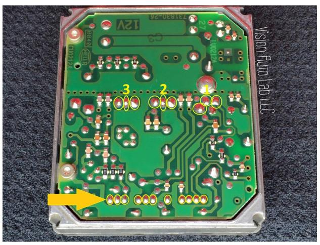
Looking from the bottom of the ballast we can see the soldering points for both the 3 MOSFETs (3 pins each) up top and the small board (10 pins) at bottom. Take not that one MOSFET has a staggered pin, this is where the ARF1405 will go.
