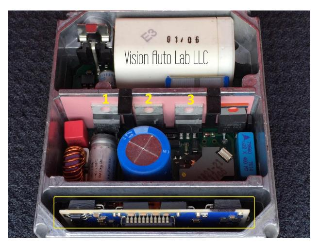
Looking at the ballast from the top you can see the 3 MOSFETs which will be replaced up top; 1, 2, and 3) along with a small perpendicularly mounted board which will be desoldered and removed from the main board.
