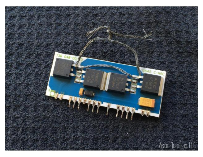
Time to desolder. I recommend starting with the board. Once the pins are free and it is ready to be pulled out thread your string or wire through the legs of the other components as shown above, The board is fragile and using string is the safest way to remove it once free. DO NOT USE PLIERS TO REMOVE THE BOARD.
