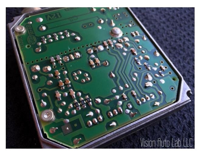
Once the 3 MOSFETs are soldered take your wire cutters and remove the excess pin length. The picture above shows the secondary board and 3 MOSFETS reinstalled and soldered in position with the MOSFET's pins trimmed.
