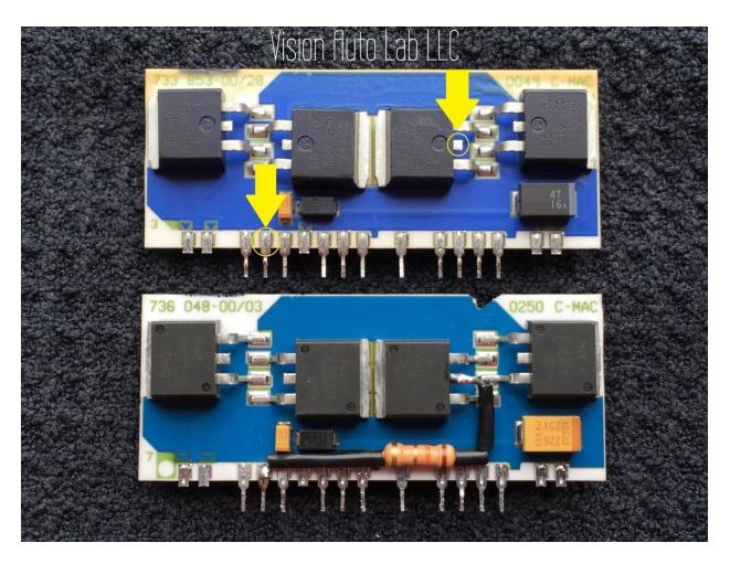
With your secondary board removed you can easily access to soldering points to add your resistor. Add your resistor to the points shown above. Take care when applying your heat shrink and make sure these is no unwanted metal-on-metal contact.
