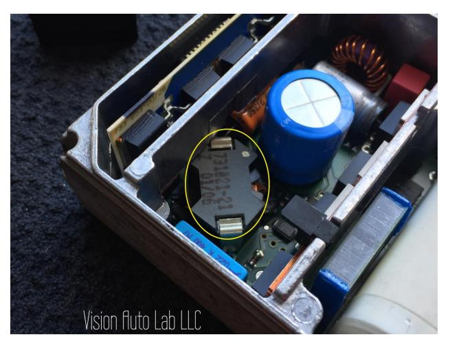
While viewing the ballast from the top, add a small amount of thermal epoxy on top of the EPCOS and install the metal heatsink.
