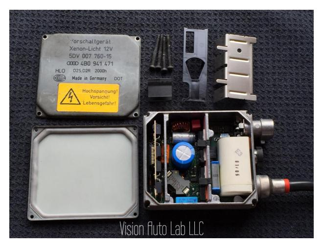
With the 2 large ballast covers removed, viewing the ballast from the top carefully remove the 3 small braces, picture above shows braces removed.
