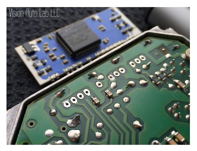
With secondary board removed clean up any excess solder and prepare the holes for reinstalling the board.
