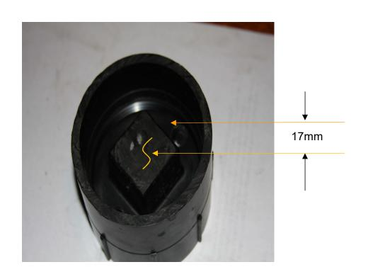
This is a 3" PVC cap with a screw-on lid. Screw in the lid inside out to match the dimensions indicated here. You can grind the PVC to the required dimensions if you need to. Put some glue on it so that the adjustments remain permanent
