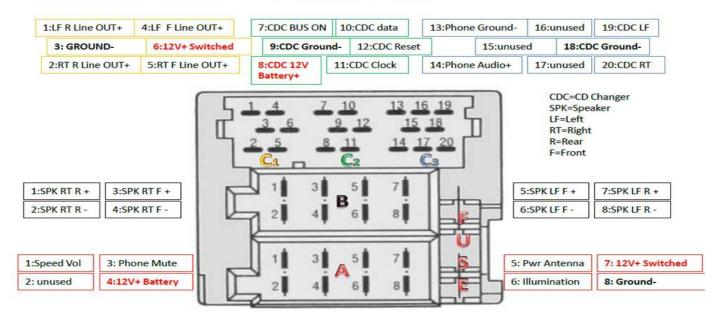
The "hi-fi" sound system has 6 speakers (2 door speakers), and all speakers are fed from the factory amp. Therefore, there is no direct connection from the radio to the speakers. The output comes out of the yellow plug and you MUST use the switched +12Vdc coming out of the new radio to power the factory amp otherwise you will have no sound.
