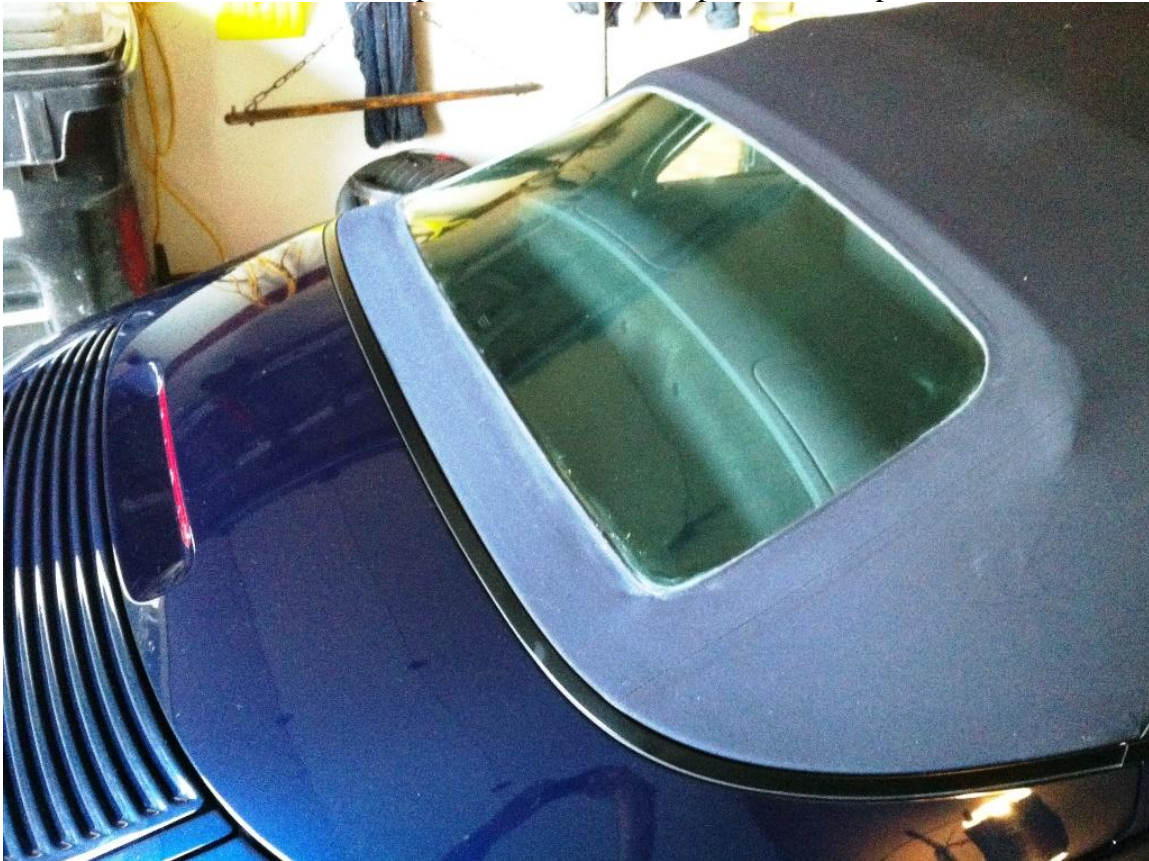
Photo 8: Completed Convertible Top Window Repair
