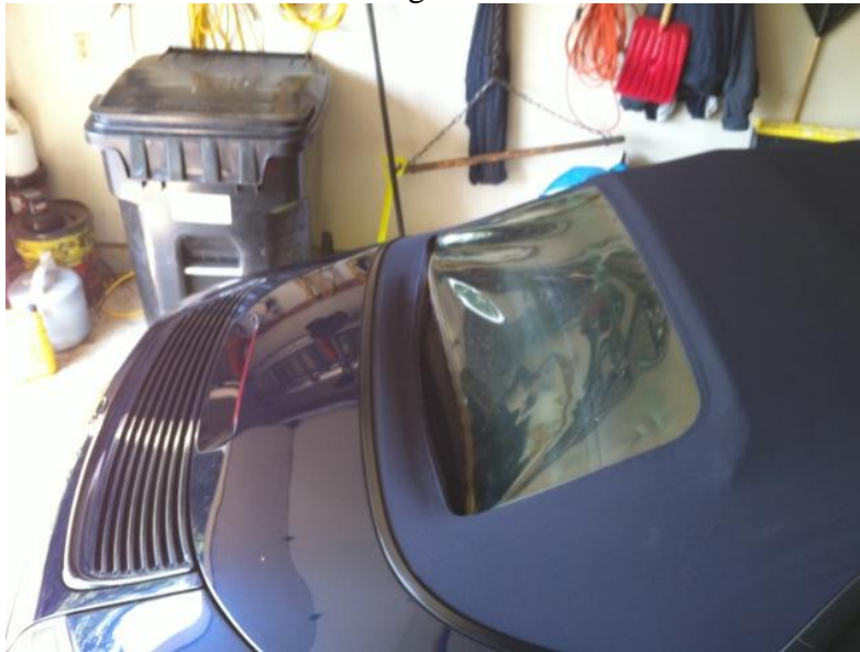
Photo 2: Window Delaminating – after a few weeks in the hot sun
