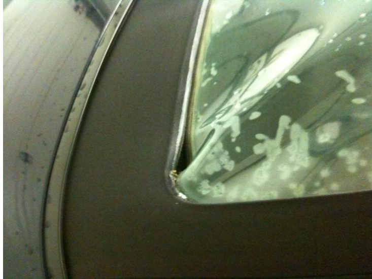
Photo 1: Window beginning to delaminate
