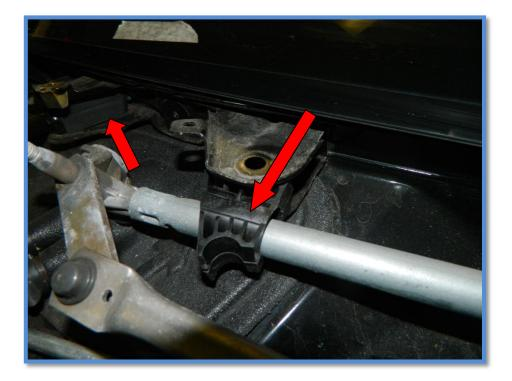
Turn over the wiper assembly, and disconnect the power connector (red) and the plastic clip (yellow).
