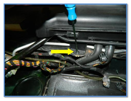
Now, when all screws removed and wires disconnected, remov the panel by puling it up from the window side (red), and pushing it toward the back of the car (yellow).
