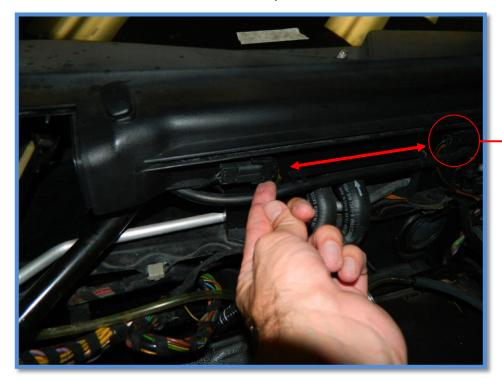
remove the screws located under the connectors (yellow) Disconnect the water line (red)
