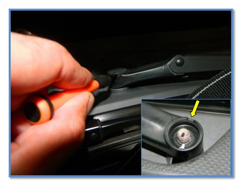
The screwdriver should be entered thru designated groove.
