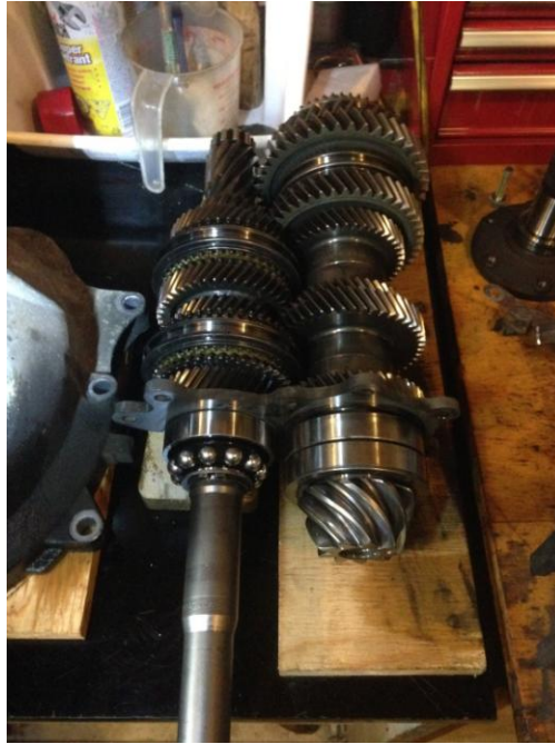
Figure 9: Gear Cluster Removed from Case
