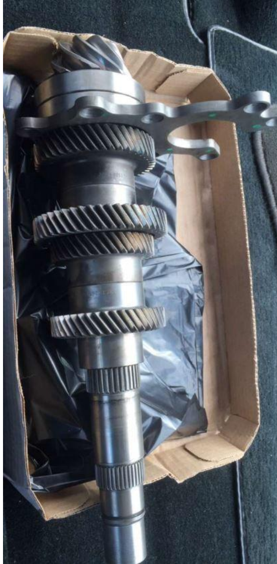
Figure 17: Counter Shaft with new Pinion Bearing
