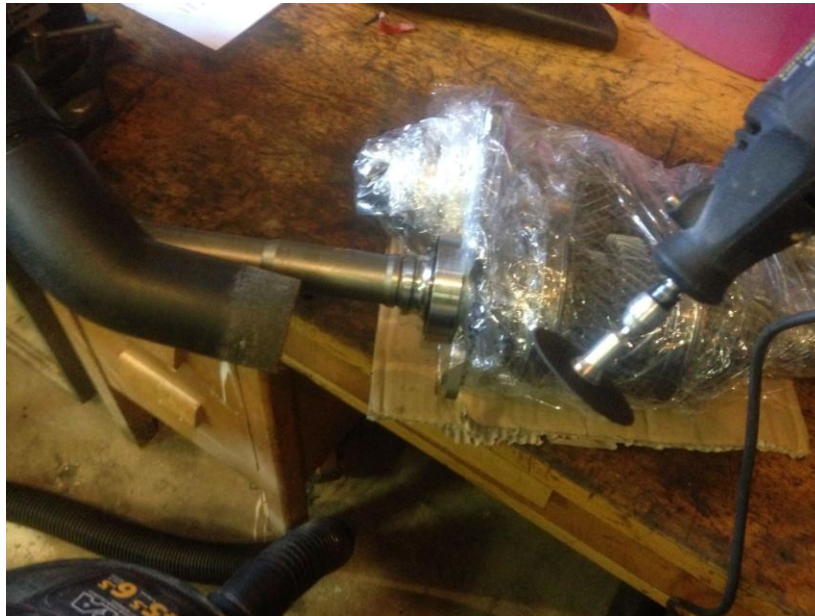
Figure 14: Cutting the Mainshaft Bearing
