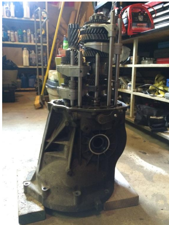
Figure 21: Shift Forks/Rods Installed
