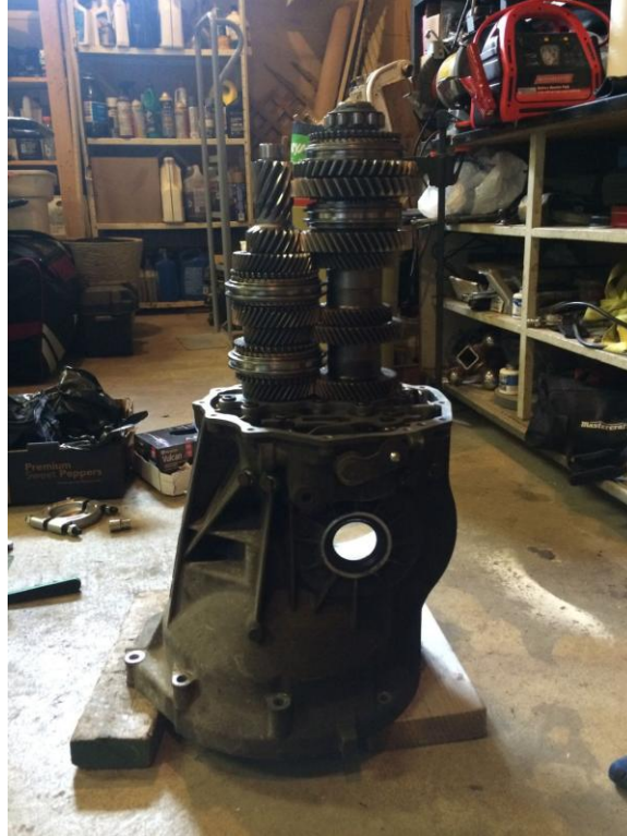
Figure 20: Gear Cluster Installed in Case
