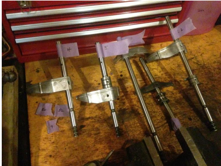
Figure 7: Shift Forks and Rods Removed
