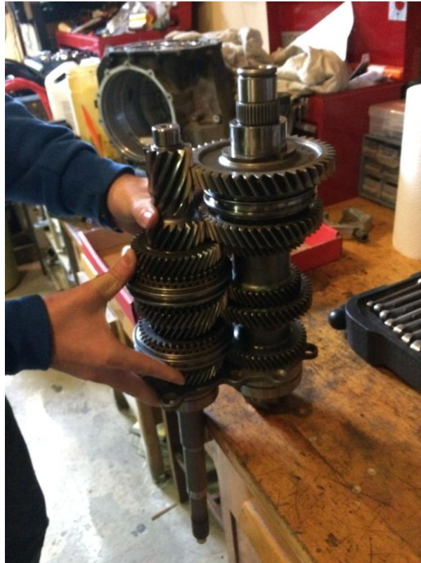
Figure 19: Stacking Components onto the Counter Shaft
