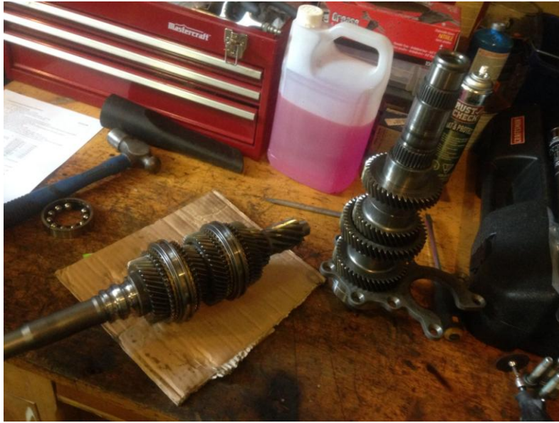
Figure 15: Mainshaft and Countershaft Separated
