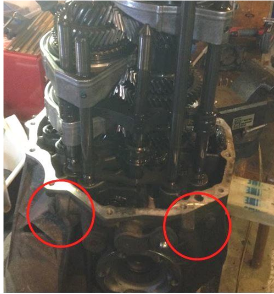
Figure 5: Shift Rod Ball and Spring Bolts
