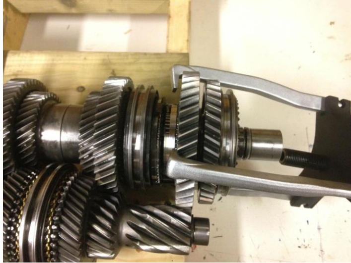
Figure 11: Pulling 1st Gear Assembly
