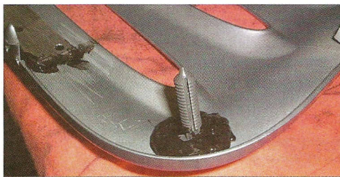
New holding pin cemented in the corner of the grill's underside leading edge...
