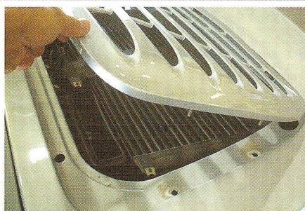
Two additional hold-down points are located on each side of the grill
