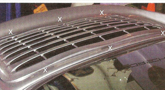
X marks the spot, or in this case, each of the hold-down pins for the grill section
