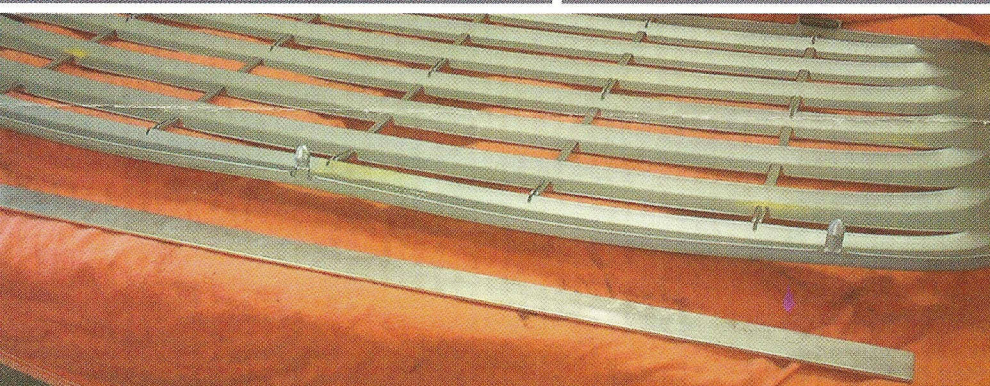
The strip of aluminum we chose to strengthen our grill was a 0.25-inch thick bar that is 1.0-inch wide and 28 inches long, seen here laying next to the grill
