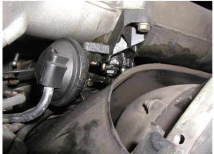
Leaking intake resonance flap with blower and ducting removed
