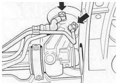
• At this point you should be able to push the rack's shaft ends in an out of the unit by hand -to the left and right as needed to clear the car's frame. I pulled off the boots before I did this step.
