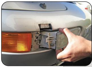
Pull fog light out of car (starting with the outboard side). You will need to pull this side hard to release the fog light from the housing.
