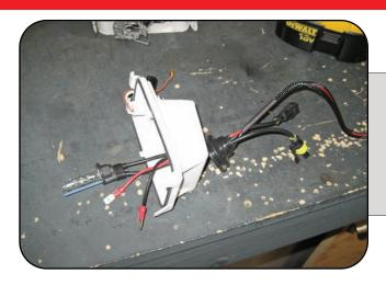
Carefully pass the H3 HID bulb and wiring through the modified fog light dust cover. The rubber grommet stays to the outside of the cover.
