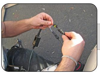
Then plug the corresponding AMP connectors from the ballast to the HID bulb.
