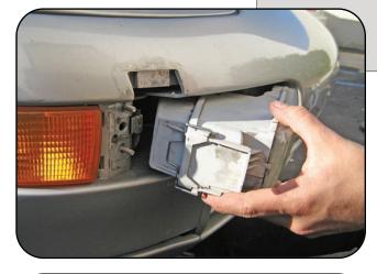
Once removed you will see 2 plugs. Remove the right plug (city lights power supply) by simply pinching down retaining clip and simultaneously pulling away from fog light.
