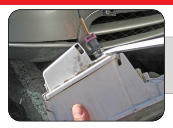
Next remove the remaining plug (fog light power supply) by opening retaining clips and simultaneously pulling away from fog light.
