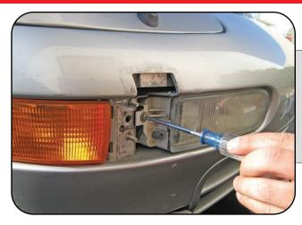
Once removed you will see a single phillips screw. Remove screw using phillips screwdriver.
