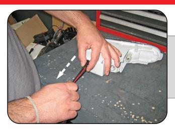
**GENTLY** pull on the wires while holding the rubber grommet firmly in place. This will eliminate any slack inside the fog light housing, giving you more wire to work with.
