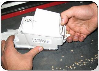
Once the fog light is removed you will be able to easily modify the housing for your new HIDs. Next remove the fog light cover retaining clip and remove cover.
