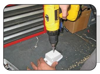
Using a drill with a Uni-bit (pictured) or a 7/8" wood spade bit drill a 7/8" hole in your low beam dust cover. This will allow you to pass the HID wiring through. **The hole must be** located DIRECTLY behind the bulb location.
