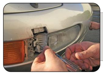
Next screw the phillips screw head back into its original location. Finally reinstall the bumperette covers using your 8mm deep socket. And replace the plastic bumperette cover over the 8mm bolts
