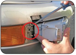
Getting the other side in is a little bit trickier. Using a flathead, move over the retaining mount (shown in photo) while simultaneously pushing the fog light into the car. It is a very tight fit which requires some muscle and finesse.
