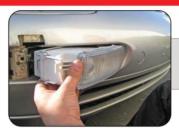
Reinstall your new HID fog light back into the bumper. Start with the side closest to the center of the car.
