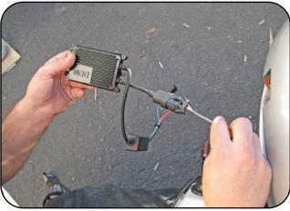
Then plug the 9006 connector on the adapter harness (the connector coming out of the fog light housing) to the ballast.
