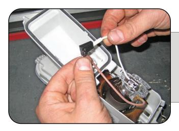
Next unplug the positive and negative female spade connectors from the fog light by pulling firmly away from the fog light bulb.
