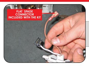
Pictured is the female spade connector crimped on properly.
