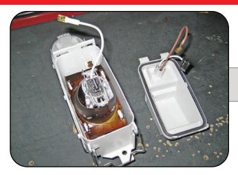
Pictured is the fog light cover/wires removed. 9
