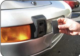
Remove bumperette cover exposing the two 8mm retaining bolts hoding the bumperette in place.
