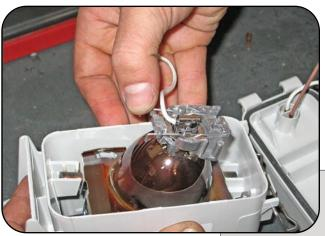
Next, pinch and release the metal retaining clips which will allows the OEM H3 fog light bulb to be removed. Then gently remove the OEM H3 bulb out of the foglight housing.
