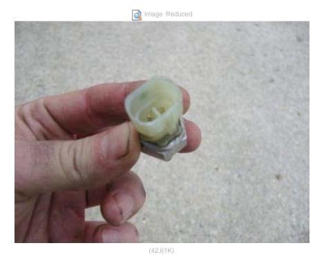
5. Reinstall the wiring connector, be sure to push it all the way in so no green rubber boot is visible, and you hear the \*click\* of the snap retainer.
