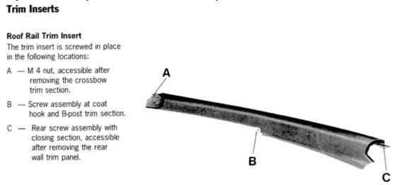
There is also some sort of sliding-into-slot thing... mine is broken from the previous owner having some loser work on it. The trim piece has to be slid backwards 40 mm to release it. Then the trim piece can be wriggled out of the car
