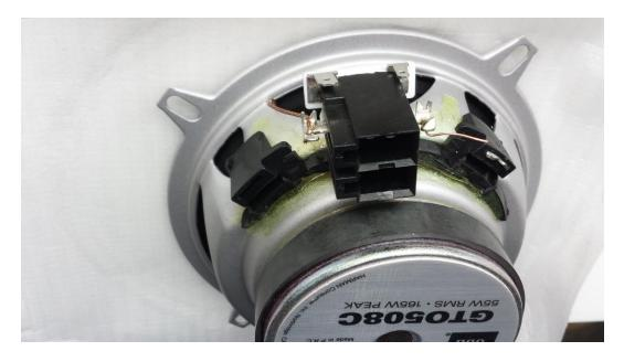
now solder the connections from the terminals on the connector to the speaker terminals. Luckily they are on the correct sides, and if you have retained enough of the connecting wires, you will save yourself a little bit of soldering. Once connected, it will look like this:
