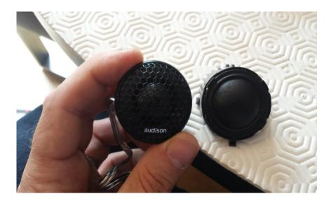
Now take the OEM tweeter unit and cut-off the connection section. Do this carefully so that you don't damage the connections and retain a small amount of plastic surround to be able to glue this back into the tweeter housing:
