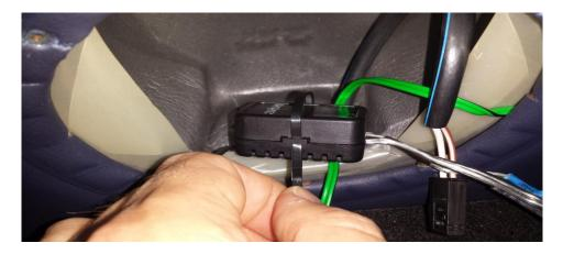
once installed, you can't see the cross over and all you have is the two connections for the woofer and the tweeter:
