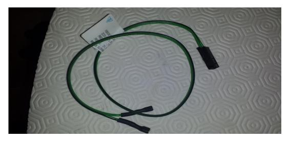
You need to produce this – remember to cover your soldering using some heat shrink:
