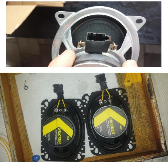
We're just dealing with a single connection here (unlike the front units), so we just need to solder on the VW connections which are the same as the Nokia's to the new Kickers: (cover the delicate parts of the speaker while soldering, because hot solder will go right through very easily) Notice that the Kickers don't protrude at all, so there's no problem refitting the original covers:
