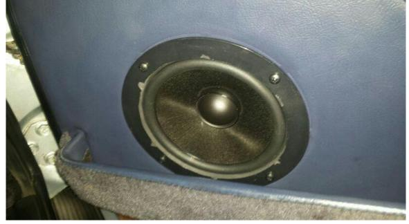
Once you have the mounting sorted for both sides, you need to go back to the Porsche OEM speakers and cut-off the dual speaker connection (it also feeds the front tweeter). Your going to attach this to your JBL upgrade speaker so that you can use the original cabling to connect it up. You want to cut-off the speaker connection in such a way that you can proceed to glue it to the new speaker as shown below:
