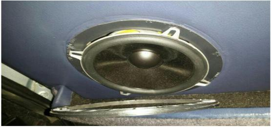
And here it's all screwed together, the standard grills can be clipped back on as normal and the movement of the speaker is not impeded because it is slightly recessed from this grill.
