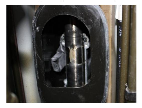
Remove the e-clip from the shift fork. This is exactly the same as the clips/washers you removed earlier. Photo below shows these clips removed. Slide the fork and shuttle half off of the shift lever.
