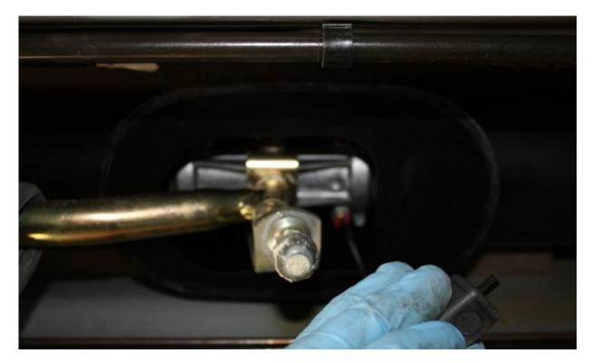
Separate the shuttle halves (this has probably already happened). Let the lower half that is attached to the shift lever/fork drop down and slip the upper half around and remove it.
