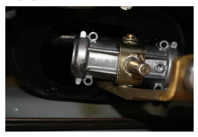
Slide the shift lever down and carefully pull from the upper rubber boot. Take this assembly to a workbench.
