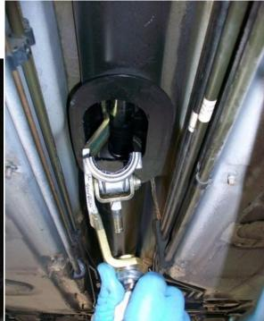
When the shift lever and shuttle half are almost in place, slip the upper shuttle half in the opposite side of the opening. The goal is to just get it up there at this point.
