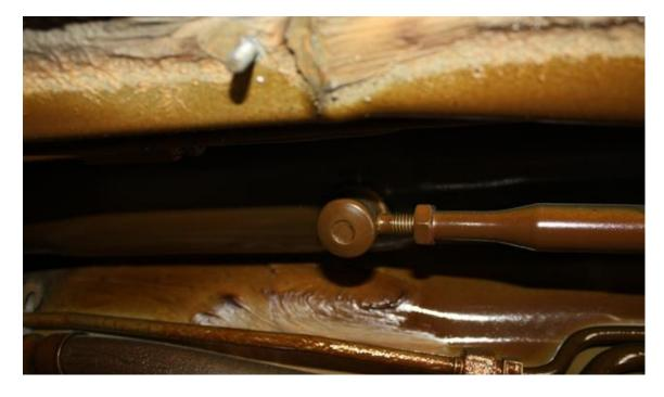
Use a small screw driver to pry off the e-clip. There will be 3 washers (2 flat and one wavy). The wavy washer is sandwiched between the 2 flat washers and keeps tension on the e-clip and bushings. Slide the shift rod and rubber boot out of the way.
