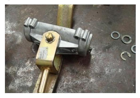
Slide the fork off of the shuttle half being careful to retain the rubber o-rings.
