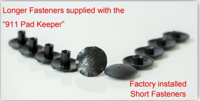
Slide the "Pad Keeper" under the Foam Pad. Starting in the middle, press the Pad Keeper upwards and line up a Body stud in an opening of the Pad Keeper, thread a Fastener on, don't tighten completely. Once all fasteners are attached, begin tightening until they are secured. Check that both ends of the Pad Keeper are seated against and under the metal drip rail. One "spare" Fastener is supplied...... \*\* Cover the Engine \*\*
