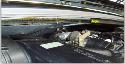
The Aluminum backed Insulation "EZ Cool" that is glued to the backside of the Pad Keeper, is Very effective in reducing sound, as well as having heat reflective properties. We found that "EZ Cool", all things being considered, was the best "Automotive" Insulation for the "911 Pad Keeper".
