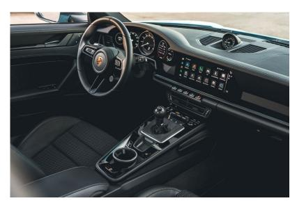
ROW YOUR OWN The 2023 Porsche Carrera T offers a three-pedal, seven-speed manual transmission as standard equipment. An eight-speed automatic transmission is a no-cost option. Cars with the automatic are equipped with a torque-vectoring mechanical rear differential. PHOTO: PORSCHE CARS NORTH AMERICA
