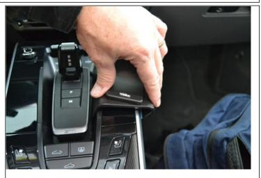
2. Press the left side of the ProClip into the opening between the shifter and the right side of the console top. Press down on the ProClip until the lower left edge hooks into the console seam.
