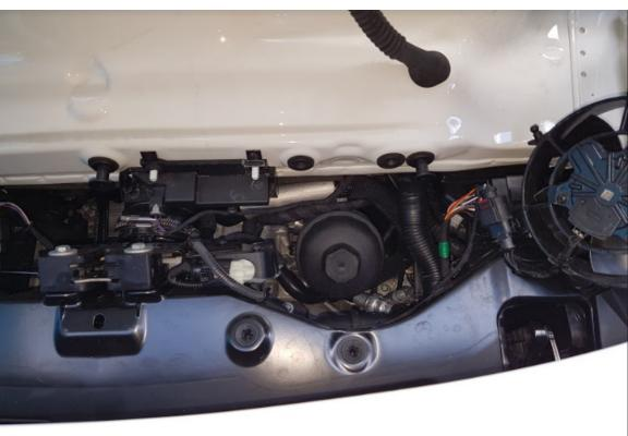
36 mm socket to remove. torque wrench ( low range ) to refit ....correct value to re install is inscribed on side of filter cover ...please check , but its a small number like  $24\ or\ 26\ Nm$  (  $18\ Lb.ft$  -ish..... )
