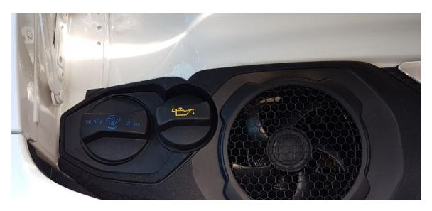
pull off cover ...( its just press fit into easy remove/re install pop mountings )
