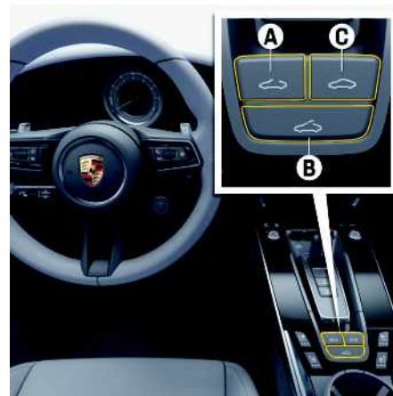
Fig. 179: Operating steel slide/tilt roof
