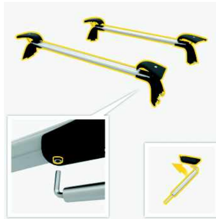
Fig. 166: Tightening the screws on the underside of the carriers
