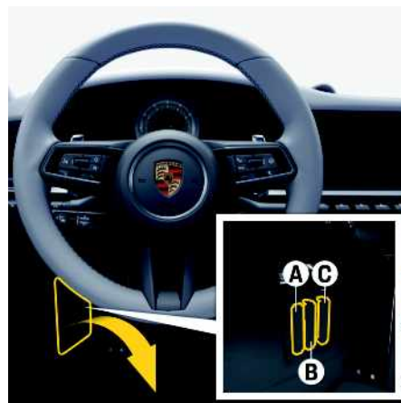
Fig. 89: Opening the fuse box in the driver's footwell
