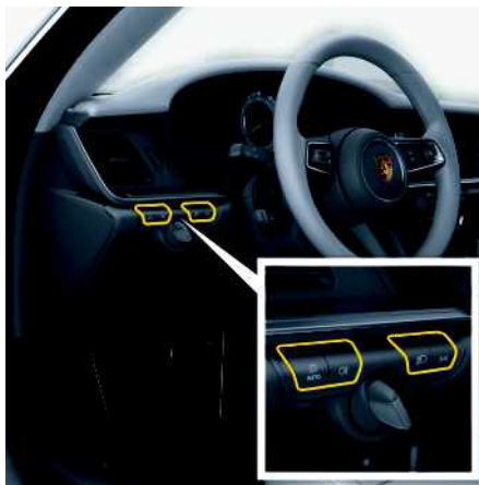
Fig. 108: Light control panel
