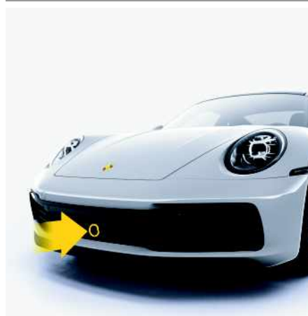
Fig. 1: Location of radar sensor
