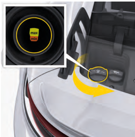
Fig. 12: Measuring the engine coolant level
