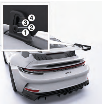
Fig. 7: Rear wing adjustment positions
