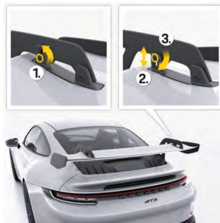
Fig. 8: Rear wing adjustment
