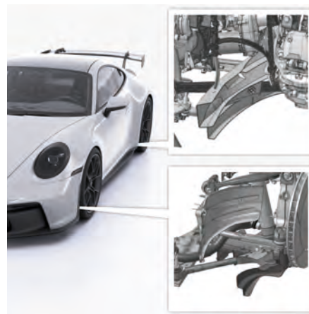
Fig. 2: Brake air spoilers and brake air ducts
