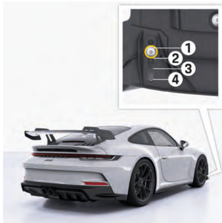
Fig. 9: Front diffuser adjustment positions
