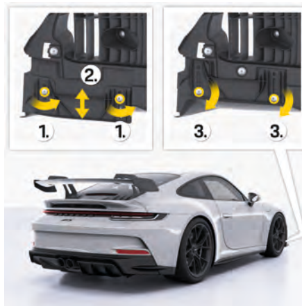
Fig. 10: Front diffuser adjustment
