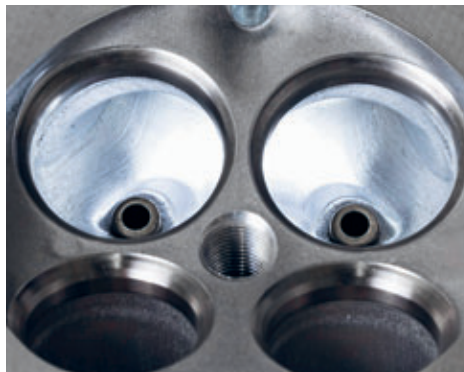
Compared to the series version (left), the intake ports of the cylinder heads in the 911 Carrera S powerkit are additionally machined and polished (right).
