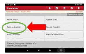
Then select the appropriate System for the Code you want to adjust (Note: This is the system listed in the pictures such as Front-end Electronics, Rear-End Electronics, Instrument Cluster or Air Conditioning)
