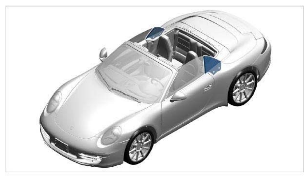
Fig 1: Identifying Rear Side Windows
