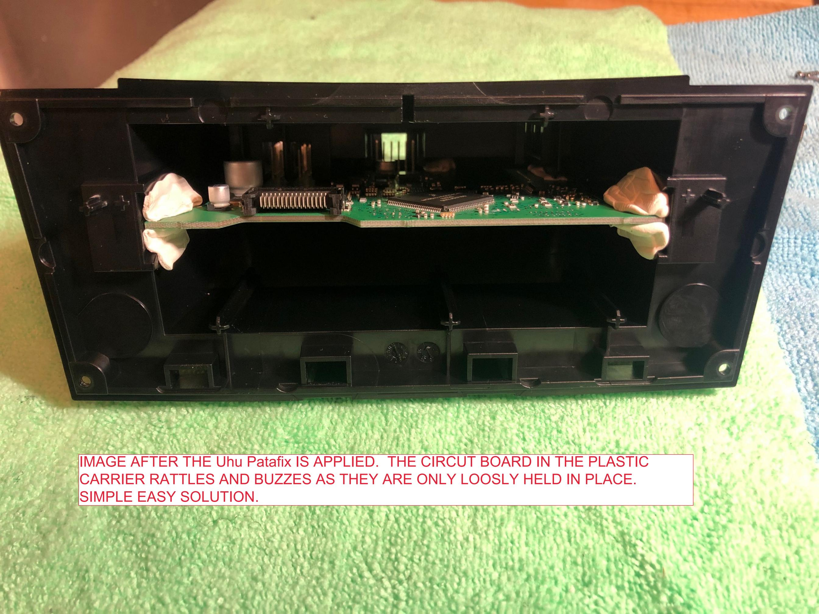
I USED THIS STUFF. IT DOESN'T DRY OUT, IT'S PERFECT FOR THE JOB. IT DOESN'T OOZE OR CREATE ANY LONGTERM PROBLEMS WITH PLASTC PARTS. IT DAMPENS VIBRATIONS AND HOLDS LOOSE CIRCUT BOARDS IN PLACE.
