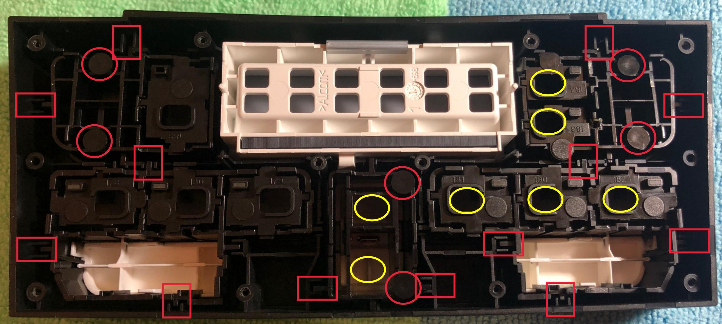
AT RED CIRCLE LOCATIONS, THESE ARE PLASTIC PINS THAT ARE VERY LOOSE AND RATTLE. THEY ACTIVATE THE BUTTON'S FUNCTIONS. FIND A THICK GREASE YOU LIKE AND APPLY A LITTLE AMOUNT ON THE SHAFT OF EACH PIN. HUGE DIFFERENCE. KILLS RATTLES!!
