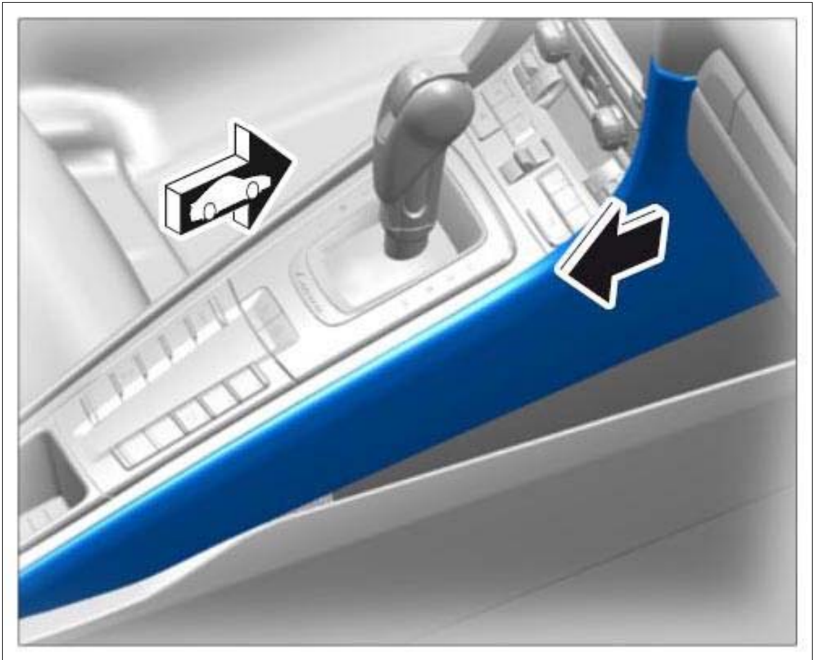
Fig 3: Removing Side Trim Panel
