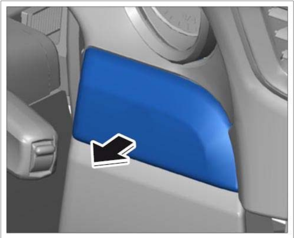
Fig 1: Removing Dashboard Molding On Driver Side (Right)
