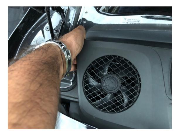
5.) Pick a fan, and grab the connector. Push the tab on the rear of the connection, and pull firmly to release the connection. There is a retaining piece to keep the fans affixed to the frame. To release, pull firm and pinch the pin from underneath. Same goes for the clip wire. Remove fan and tuck the clip away from the opening. Repeat for the other fan. Make sure you note which fan is right and left.
