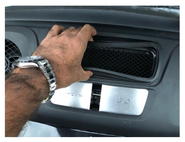
4.) Pull on the top edge of the plastic cover to free from top corner retaining plugs. Once free, repeat with bottom corner plugs. Once loose, shift up and lift out, exposing the fans and their connector pieces.
