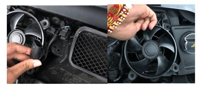
6.) To remove the plenum, first unhook the release cable from its seat on the plenum. Then, firm lift on the plenum, releasing the pressure holds from the interior plumbing. Lift out completely from bay.
