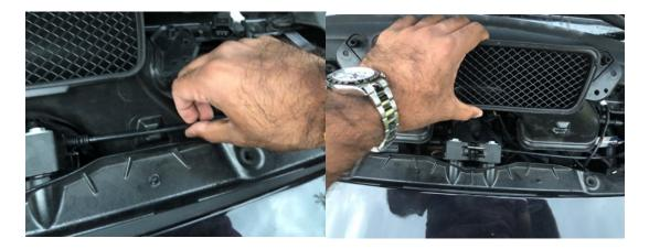
7.) Note position of the Y-pipe sensor. Practice releasing and installing the connector with 1 hand. Get a feel for how the plug releases and the behavior of the plug when properly inserted.
