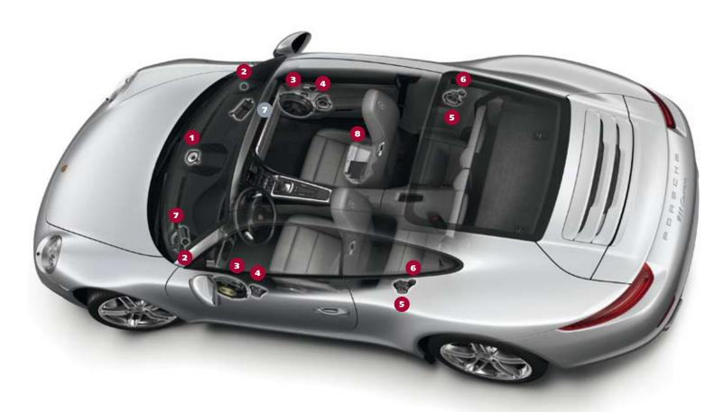
Each part of the Bose sound system has been carefully engineered to work with the others for better performance. Replacing the factory-installed Porsche Communication Management (PCM) or CD-Radio (CDR-30) or any other sound system component can significantly reduce system performance. Bose system components and their respective locations are identical in the Porsche 911 Carrera (S) Cabriolet. The equalisation is customised to the specific acoustical properties of the cabin.
