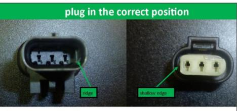
• The plug must be as show on the picture will be with the shallow edge on the side of the ridge.
