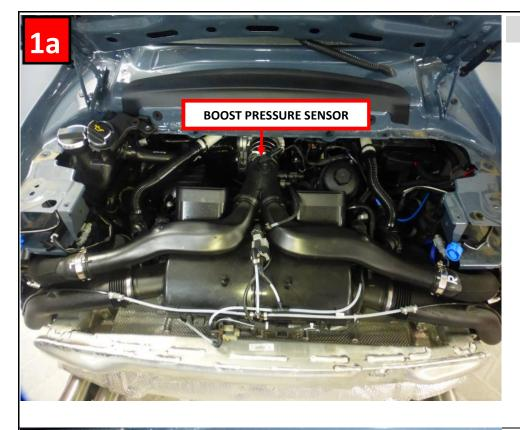
The boost pressure sensor is located at the central point of the air supply.
