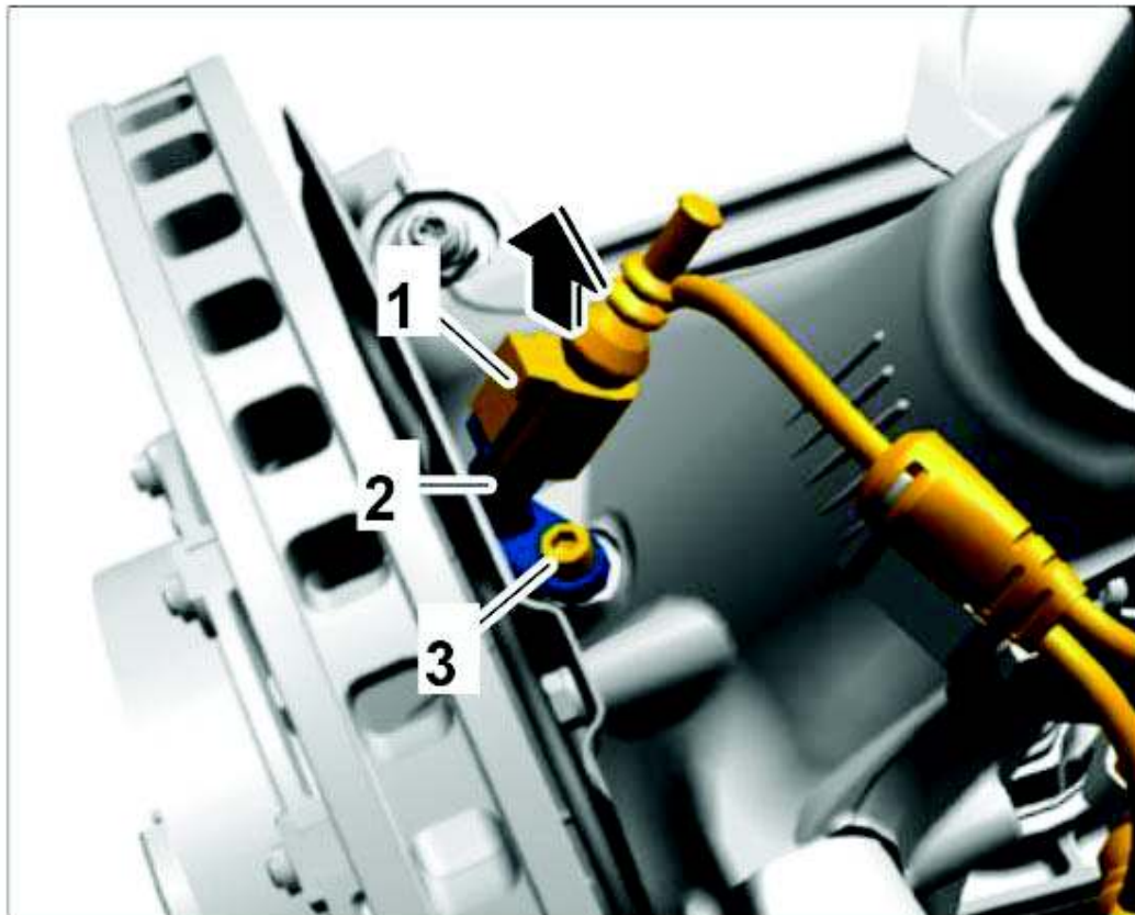
Fig. 1: Releasing Electric Plug Connection From Speed Sensor Courtesy of PORSCHE CARS NORTH AMERICA, INC.
