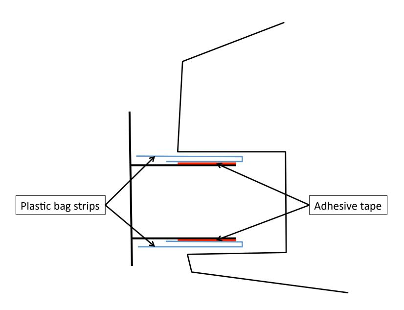
Note: clearance between bracket and inside of vent exaggerated
