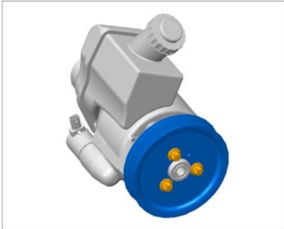
Fig. 50: Identifying Pump Pulley
