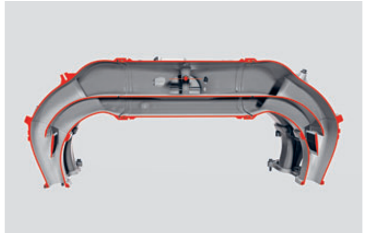
Improved torque curve in partial load operation: The cast aluminum intake system has a tuning flap in the receiver volume that enables separation of the two cylinder banks.
