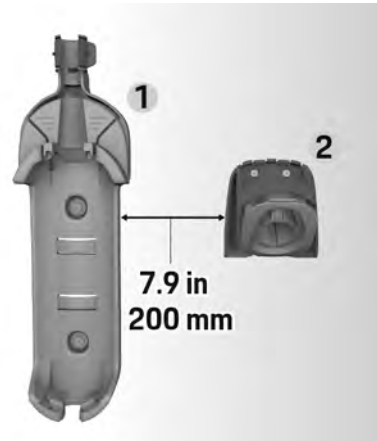
Fig. 2: Distance from wall mount to plug holder
