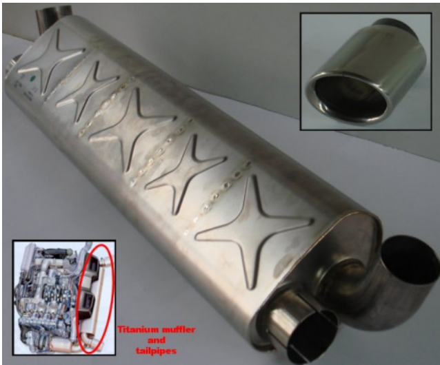
Fig. 2. Porsche 911 GT2 titanium muffler and tailpipe
