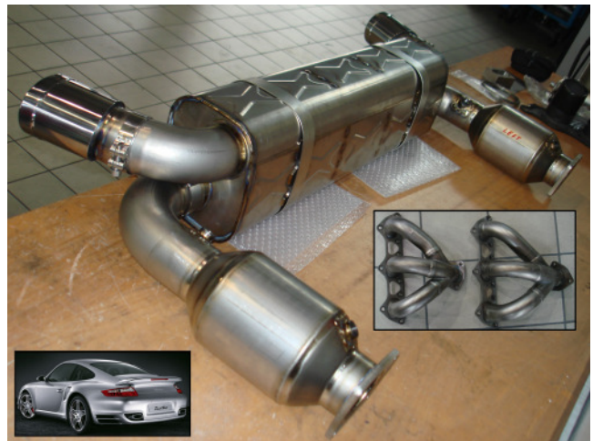
Fig. 3. Porsche 911 Turbo complete titanium exhaust system
