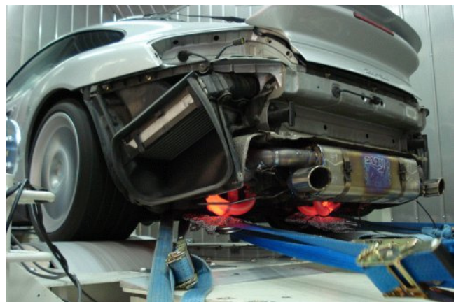
Fig. 4. Performance test of the Porsche 911 Turbo on a car dynamometer
