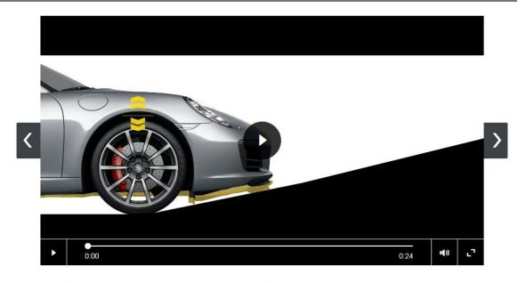
Hydraulic function for raising the front axle by approximately 1.5 in. at the push of a button to increase ground clearance at speeds of up to 37 mph.
